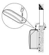
The external unit may be installed above or at the same height as the internal unit, on the condition that the difference is no more than  $5^{"}$  (1.5 m.) The suction and air-delivery portions of external unit must not be blocked by obstacles of any nature. The distance between the back of the appliance and the wall must be six 2  $1/2^{"}$  (6) cm.
